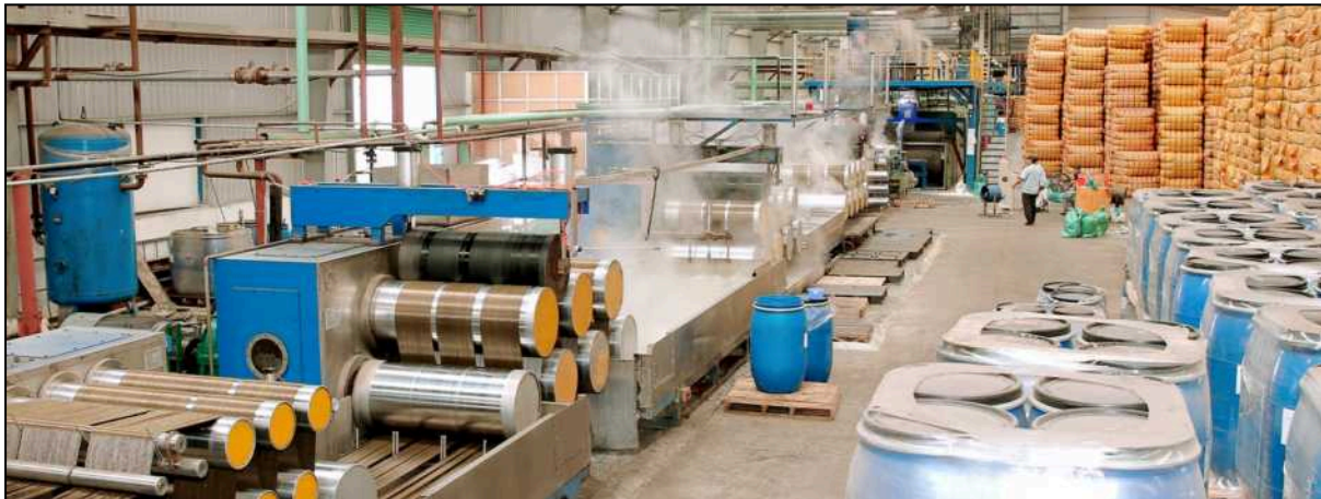
Figure 12: An image showing machinery during the process of stretching plastic into fibre (Source: Mekong Fibre)
