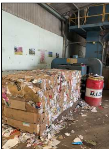
Figure 15: An image displaying the bales of paper waste released from the baler post-compression
