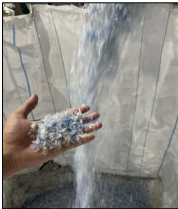
Figure 25: An image of the PET flakes post coldwater cleaning, separation from non-PET plastics, warm water cleaning and chemical treatment.
