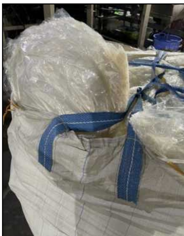
Figure 26: Image of the PET plastic sheets
