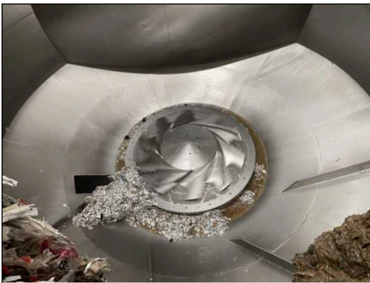
Figure 19: Container used for separating paper from other materials after the process is complete
