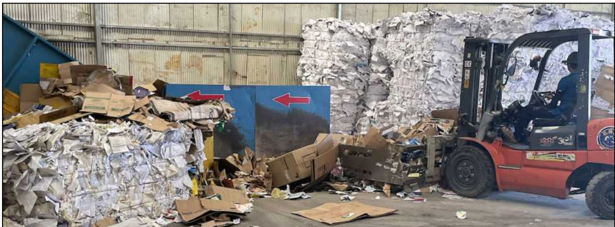
Figure 14: An image showing a worker at Bao Ngoc UBC/ Paper Collector inputting paper waste into a baler for its compression
