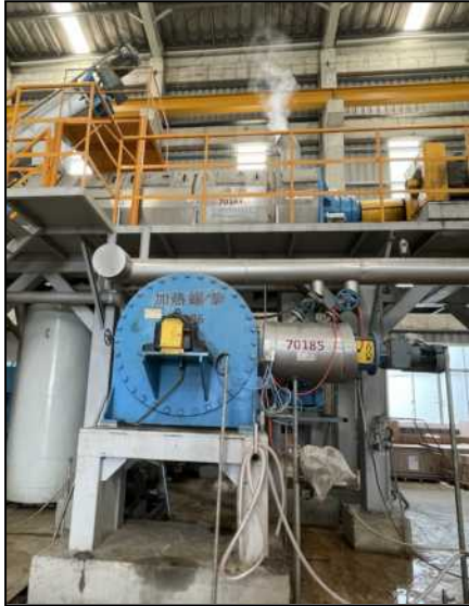
Figure 21: A machine adding heat and pressure to create paper powder
